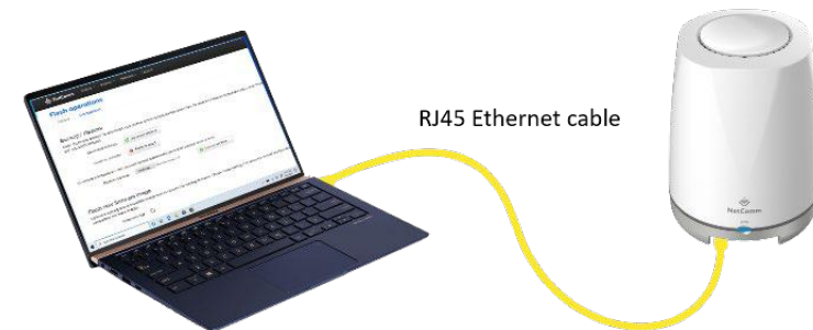
Figure 7 – RJ45 Ethernet cable connecting PC with NS-01
