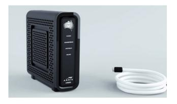
3. Ensure power is connected to the nbn® Connection Box. The POWER, DOWNSTREAM, UPSTREAM and ONLINE lights should be on.
