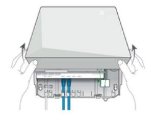
3. Ensure that the power cable is securely in place and that the Power and Optical lights are showing as steady green on the nbn® Connection Box.
