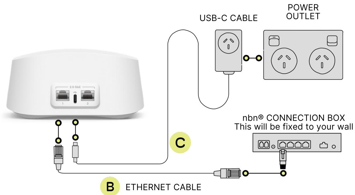
**IMPORTANT:** You will need to plug the ethernet cable from your eero 7 into your Network Termination Device's activated Uni-D port. If you are unsure which port has been activated, check your nbn® Ready to Go email from us.
